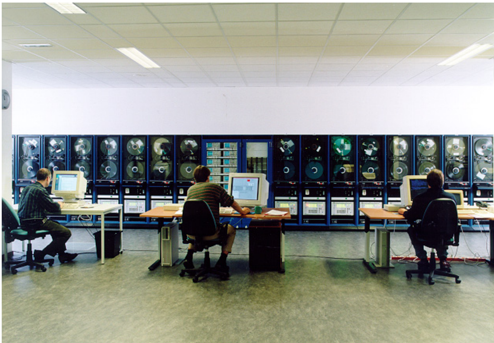
16-station VLBI correlator at JIVE in The Netherlands
